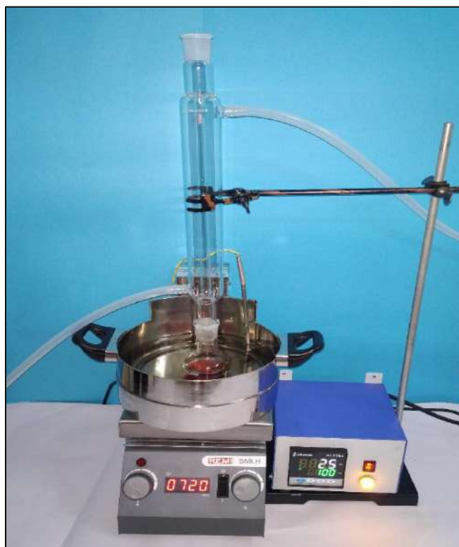
Figure 2.1: Schematic depiction of reflux condensation assembly
