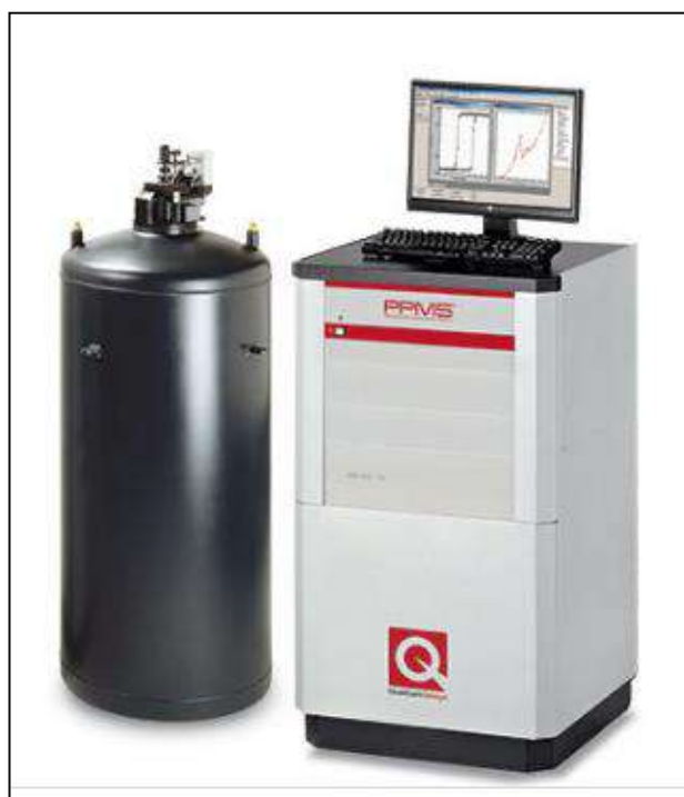
Figure 2.12: Digital photograph of vibrating sample magnetometer ( https://qdusa.com/products/ppms.html )
