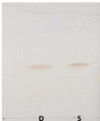
Fig. 4.4.1: TLC profile showing separation of purified secondary metabolites on Silica gel TLC plate where, S-standard diosgenin, D- purified diosgenin
